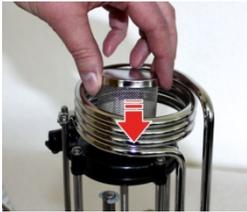
12. **Dry the unit carefully** to prevent the ingress of moisture into the interior. After having cleaned the unit install the particle filter and the protection grid in reverse order.
