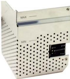
Fill the bath tank with softened/decalcified water. Observe the minimum and maximum filling height according to the marks on the protection grid.
