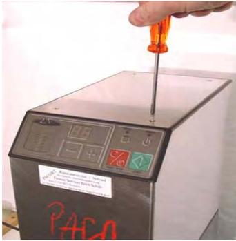
**Remove** metal top plate (4 screws)
