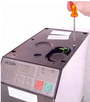
**Remove the 6 sunken screws
